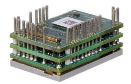
The FXE060-25-EM is a FlexPro® series Extended Environment servo drive with IMPACT™ architecture.
