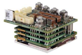
The **FM100-50-EM** is a single-axis servo drive and integration board assembly for a FE100-50-EM FlexPro<sup>®</sup> series servo drive with IMPACT<sup>™</sup> architecture. Connections to the controller, motor, power, and feedback are simplified through the standard connectors featured on the board.
