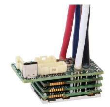
The **FM060-45C-EM** is a single-axis servo drive and integration board assembly for a FE060-45C-EM FlexPro® series servo drive with IMPACT<sup>TM</sup> architecture. Connections to the controller, motor, power, and feedback are simplified through the standard connectors featured on the board.
