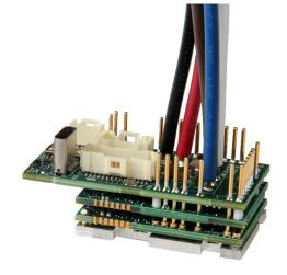
The **FM060-25-RM** is a single-axis servo drive and integration board assembly for a FE060-25-RM FlexPro® series servo drive with IMPACT<sup>TM</sup> architecture. Connections to the controller, motor, power, and feedback are simplified through the standard connectors featured on the board.
