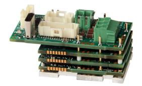
The **FM060-1-EM** is a single-axis servo drive and integration board assembly for a FE060-1-EM FlexPro® series servo drive with IMPACT<sup>TM</sup> architecture. Connections to the controller, motor, power, and feedback are simplified through the standard connectors featured on the board.
