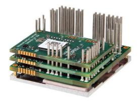
The **FE100-50-IPM** is a FlexPro® series servo drive with IMPACT™ architecture.
