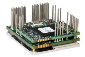
The **FE100-50-CM** is a FlexPro® series servo drive with IMPACT<sup>TM</sup> architecture.
