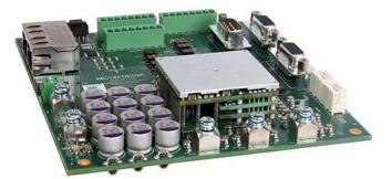
The FD100-50-RM is a servo drive and development board assembly for a FE100-50-RM FlexPro<sup>®</sup> series servo drive with IMPACT<sup>TM</sup> architecture. Connections to the controller, motor, power, and feedback are simplified through the standard connectors featured on the board. The FD100-50-RM is ideal for prototyping and can be used in production and industrial environments as well.
