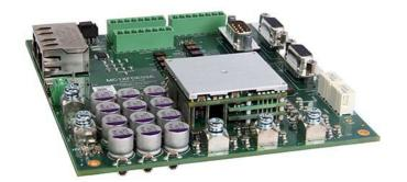
The **FD100-50-IPM** is a servo drive and development board assembly for a FE100-50-IPM FlexPro<sup>®</sup> series servo drive with IMPACT<sup>TM</sup> architecture. Connections to the controller, motor, power, and feedback are simplified through the standard connectors featured on the board. The **FD100-50-IPM** is ideal for prototyping and can be used in production and industrial environments as well.
