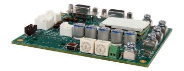
The **FD100-25-RM** is a servo drive and development board assembly for a FE100-25-RM FlexPro<sup>®</sup> series servo drive with IMPACT<sup>TM</sup> architecture. Connections to the controller, motor, power, and feedback are simplified through the standard connectors featured on the board. The **FD100-25-RM** is ideal for prototyping and can be used in production and industrial environments as well.
