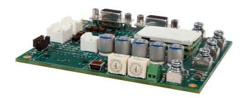
The **FD060-60C-RM** is a servo drive and development board assembly for a FE060-60C-RM FlexPro<sup>®</sup> series servo drive with IMPACT<sup>TM</sup> architecture. Connections to the controller, motor, power, and feedback are simplified through the standard connectors featured on the board. The **FD060-60C-RM** is ideal for prototyping and can be used in production and industrial environments as well.
