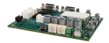
The **FD060-60C-CM** is a servo drive and development board assembly for a FE060-60C-CM FlexPro<sup>®</sup> series servo drive with IMPACT<sup>TM</sup> architecture. Connections to the controller, motor, power, and feedback are simplified through the standard connectors featured on the board. The **FD060-60C-CM** is ideal for prototyping and can be used in production and industrial environments as well.
