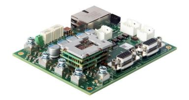
The **FD060-5-EM** is a servo drive and development board assembly for a FE060-5-EM FlexPro<sup>®</sup> series servo drive with IMPACT<sup>TM</sup> architecture. Connections to the controller, motor, power, and feedback are simplified through the standard connectors featured on the board. The **FD060-5-EM** is ideal for prototyping and can be used in production and industrial environments as well.
