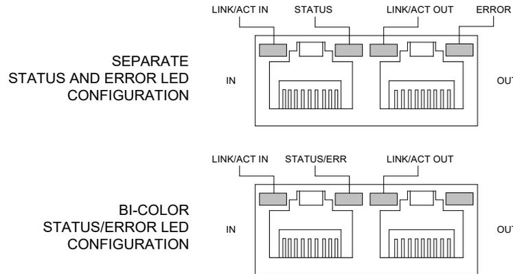
LINK/ACT IN and LINK/ACT OUT are used to drive the corresponding LINK IN and LINK OUT LEDs on a typical RJ-45 connector. The two STATUS/ERR pins are used to drive a bi-color Status LED or two separate single-color LEDs, depending on the user configuration (reference the DZEANTU Hardware Installation Manual for the recommended wiring diagram, available for download at [www.a-m-c.com](http://www.a-m-c.com)). The LED Function Protocol tables below describe typical LED functionality.
