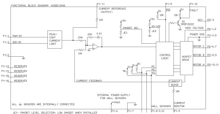
JE1- INHIBIT LEVEL SELECTION: LOW INHIBIT WHEN INSTALLED LOW ENABLE WHEN NOT INSTALLED
