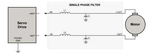
NOTE: Capacitor is not used on all models. See Specifications above for applicable capacitance values
